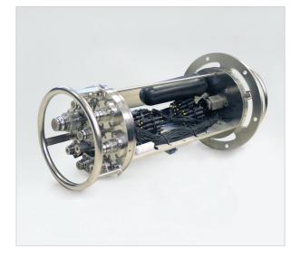
The TrustLink API FITA is a unique subsea connectivity system that assembles a harness cable or array of harness cables to a single cable, typically linking critical subsea control systems to an umbilical. Unlike other termination assemblies, the FITA can be assembled on site without the need for moulding.
