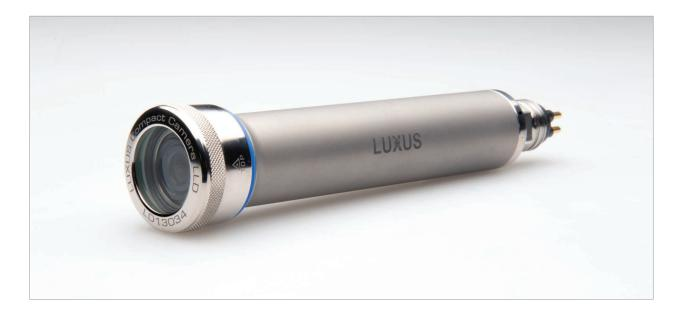
The LUXUS compact long line driver camera is a LUXUS compact camera fitted with a video signal amplifying unit. This unit increases the signal and compensates losses when the camera is used with extensive cable lengths for applications that do not involve telemetry.
