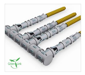
MacArtney GreenLink hubs are heavy-duty, dry-mate modular 'subsea sockets' made up to house multiple cables. Each module is mechanically linked to other modules using GreenLink inline termination technology. Extra sections can be added at initial launch or at a later stage, making the GreenLink hub a flexible option over time.
