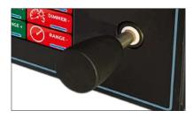
The joystick can be used to move the searchlight in MANUAL mode
