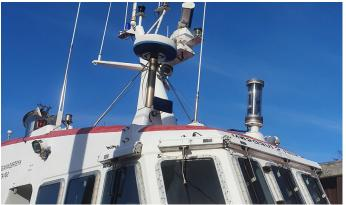
Searchmaster Searchlight keeps the focus on the distressed and makes it possible to perform fast and accurate rescue operations without occupying the crew.
