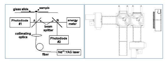
Description: The LITF-01 Laser Ignition Test Fixture is designed to test ignition threshold and delays of laser initiated energetic material.
