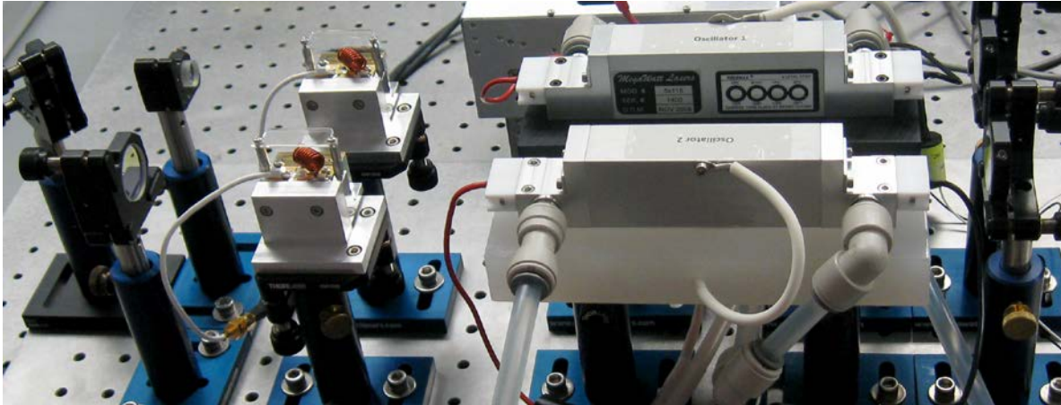
Dual Configuration of 200mJ Q-switched Laser
